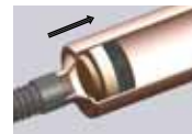
Snap disks operate and close the device, stopping heat transfer into condenser
